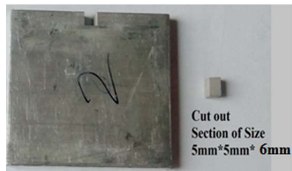
Fig. 2. Aluminium work piece after machining
